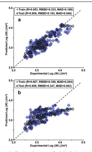
**Figure 6** Experimental versus predicted liquefaction capacity energy using the LGP correlations. (a): Eq. (7); (b): Eq. (8).
