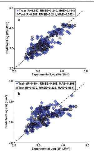
**Figure 7** Experimental versus predicted liquefaction capacity energy using the MEP correlations. (a): Eq. (9); (b): Eq. (10).
